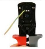
Choose the adapter head (sold separately), keep vertical and slide it into the handle until the mechanical end.
