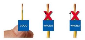
Position the contact in the bottom of the tool by checking its orientation.
