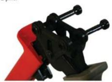
3) Close the two pins simultaneously to maintain the head.
