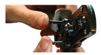
Place conductors, with no deteriorations, in the bucket contact.
