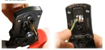
To control crimp quality, slighty pull cable with two fingers to control retention.
